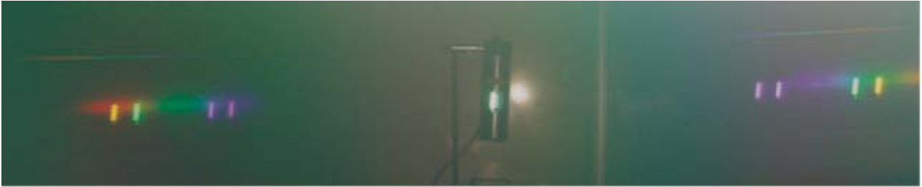
Figure 3: The first order diffraction spectrum (to left and right) produced by viewing a mercury discharge lamp (centre) through diffraction spectacles.
